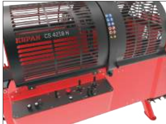
KR PAN CS 4218 H with manual hydraulic control levers
