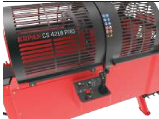
KR PAN CS 4218 H with manual hydraulic control levers
